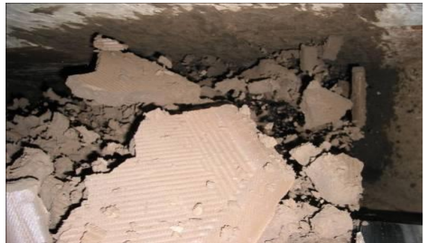
Mechanical dewatered sewage sludge (38 % DS), out of a Chamber Filter Press
