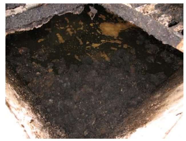
High energy content, highly viscose Sludge, in a Receiving Hopper at an Artificial Fuel Treatment Facility of a Cement Plant.
